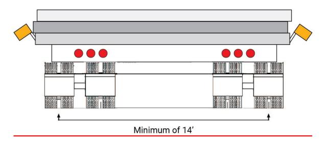
004.01B A Single Trip Permit may be issued for construction equipment that is driven on the road, provided it is equipped with flotation tires that do not exceed the limits for individual tire specifications. The individual tire sizes will be required by the Department for permit issuance and will be placed on the permit.
